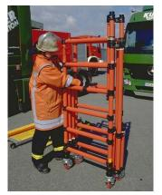
Unlock the brakes of the swivel castors
