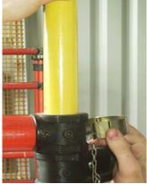
6. Release the safety clip, set the handrail to the requested height, push the safety clip in for locking
