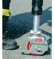
7. Block the swivel castor or check the base plate for secure stand
